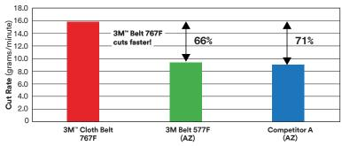
\* Results based on an automated, 54 minute grinding time backstand test on 1045 steel using 36" long belts, grade 36 and grade 36+.
